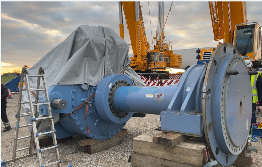
Figure 46: Main Bearing and Shaft Refurbishment at Twin Rivers
