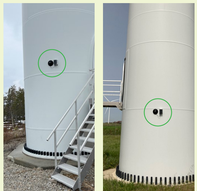
Figure 11: PING acoustic devices installed on turbine towers at Trattberget (left) and Arlena & Tessennano (right)
